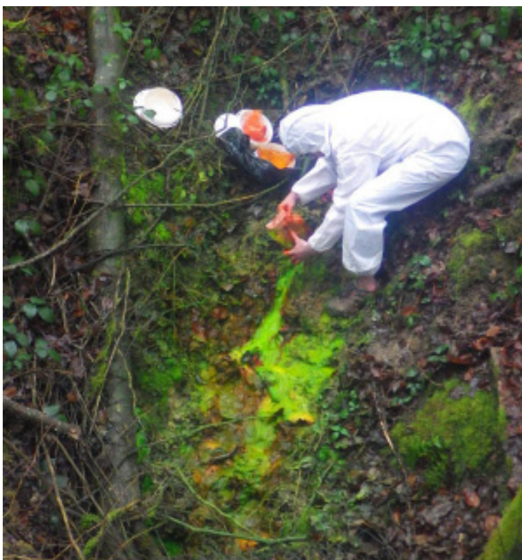
Injection de la fluor  c  ine...
